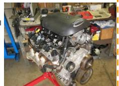
Unlike some of the Gen IV engines it does not have displacement on demand or variable valve timing. The Gen IV engines use a 58 tooth crank trigger and require a different wiring harness and computer. The LS2 and the LS4 are Gen IV engines.
