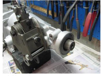
The original '63 and a half, '64, and '65 Muncie transmissions had a smaller 7/8 inch diameter counter shaft that the cluster gear in the bottom of the transmission rotates on. The transmission was beefed up starting with the '66 model year and all the later transmissions have a 1 inch diameter counter shaft. The '63 thru '70 transmissions used a 27 spline output shaft. The '71 thru '74 transmissions used the 32 spline output shaft.
