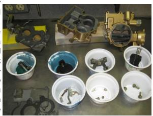
Rochester 2GC carburetors were also used on boats. Some Merc Marine 2GCs used a spring loaded needle and seat. I haven 't tried this yet but it could help prevent a float sticking, especially on and end carb that may not get dumped in all the time.
