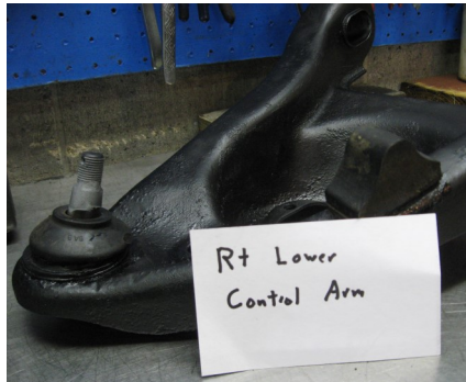
Notice Dried, Cracked, Bushings
