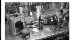
Muncie 4 speed transmissions rebuilt for \$275.00 labor, parts extra. The basic rebuild kit consists of front and rear bearings, all needle bearings, gaskets, snap rings, seals, synchro rings, front input retainer nut, synchro keys and springs. Also includes new counter shaft. My cost on the overhaul parts kit is \$126.00 plus ship-
