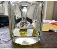
Working on vintage car brakes today. Couldn't decide if it had silicone brake fluid or conventional brake fluid. You cannot mix them. Siphon some of the brake fluid out of the master cylinder and put it in a jar with water. See the picture with the can of brake fluid in it? Since conventional brake fluid is hydroscopic, it mixed completely. The bottom picture is silicone brake fluid and water and you can see it did not mix. This particular car did have
